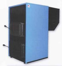
This single feeder anthracite stoker furnace is the right choice if you are looking to heat a home up to 3500sq/ft. The internal heating surface is approximately 26 square feet, which consists of 18 tubes transferring more of the heat from inside the furnace to your home where it belongs instead of up the chimney. This model comes standard with a 200 lb. hopper. Optional Cold Air Return Plenum with 20" X 20" Filter.
