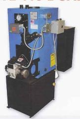
A two piece boiler designed with our Pocono coal stoker feeder as a base unit. The pressure vessel/ oil burner unit sits on top and is manufactured by Axeman-Anderson. It Can also be fitted with a Natural Gas or Propane burner for additional charge. The WL-110 burns Rice-sized or Buckwheatsized Anthracite Coal. Optional Flue Clean out and 5GPM DHW Coil.
